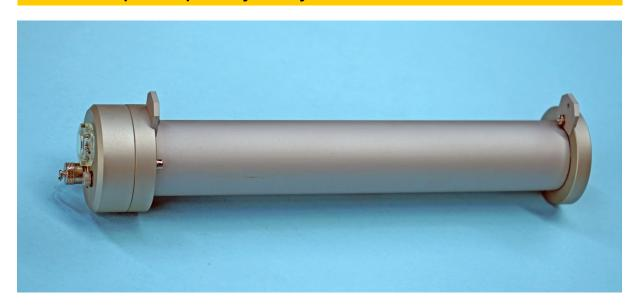
The Middleton Solar DN5-AF is a precision pyrheliometer for measuring the solar Direct Normal Irradiance (DNI) when aimed at the sun. It exceeds the International Organization for Standardization (ISO) specifications for a Fast Response Spectrally Flat Pyrheliometer of Class A. The DN5-AF has a compact thermopile sensor embedded in an integrating cavity, with the sensor not directly exposed to the sun to achieve very low zero off-set. The DN5-BF is a Class B version of the DN5-AF.
