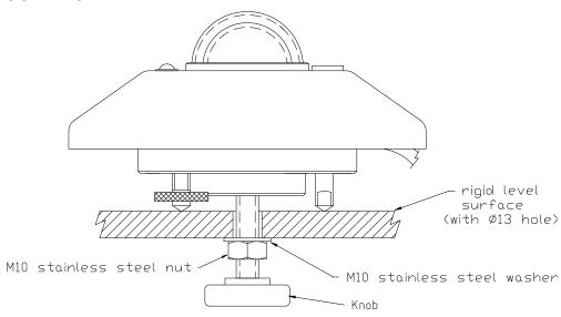
The EQ09-A should be mounted on a rigid level surface. The instrument has a central M10 x 1.5p hole in its base. The mounting knob supplied should be screwed into this hole and the instrument mounted, as shown above, using the washer & nut provided. Adjust the height of the feet so the circular level is centred. Secure the knob & nut finger-tight only (do not over-tighten).
