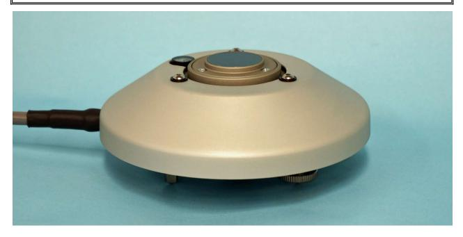
The Middleton Solar PG01-E Pyrgeometer is for measuring long wave radiation emitted by the atmosphere (downwelling) or the Earth surface (upwelling). It uses a passive thermoelectric sensor shielded by a flat silicon window. The window is coated to exclude radiation below 4.5  $\mu$ m. The PG01-E has in-built signal amplifier. It is sealed and fully weatherproof.
