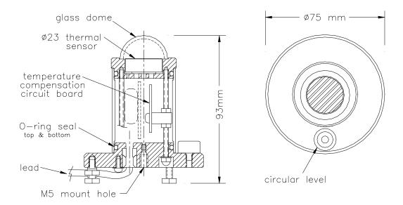
Meets the ISO 9060:2018 specifications for a Spectrally Flat Pyranometer of Class B, and the equivalent WMO specifications for a Good Quality Pyranometer.
