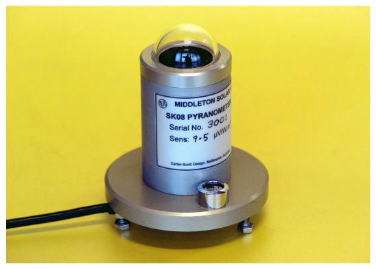
The Middleton SK08 is a solar pyranometer for the accurate measurement of Global Horizontal Irradiance (GHI) on a plane surface. It exceeds the ISO specifications for a Class B pyranometer. The SK08 features a passive thermoelectric sensor, optimised for thermal stability. The SK08-E version has an inbuilt signal amplifier.
