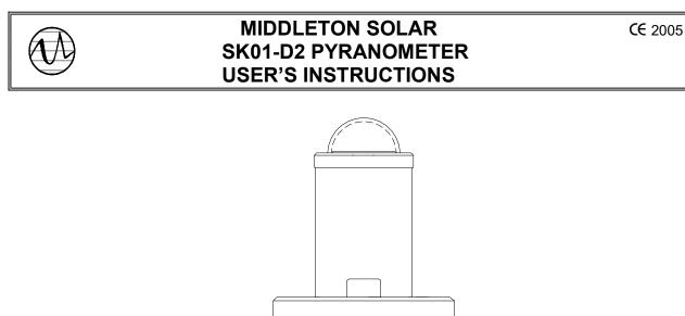
The SK01-D2 pyranometer is for measuring solar global radiation. It uses a silicon photodiode detector shielded by a cosine corrected diffuser and has a glass dome to keep debris off the diffuser. It is sealed and fully weatherproof. The detector signal is boosted by a low noise amplifier that is drift stabilised.
