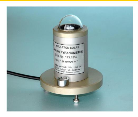
The SK01-D2 is a simple pyranometer for measuring total solar global radiation on a horizontal surface. The SKO1-DP2 version incorporates a special filter to limit its sensitivity to the Photosynthetically Active Radiation region of the solar spectrum (400-700nm).
