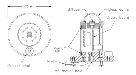
In-built signal amplifier to give a millivolt output for easy measurement.
