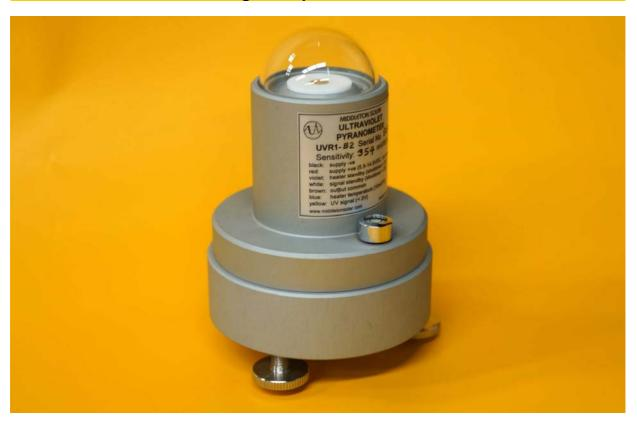
The Middleton Solar UVR1 series are precision filter radiometers for measuring solar global ultraviolet irradiance. The UVR1-T2 and UVR1-A2 are suitable for air pollution monitoring. The UVR1-B2 is suitable for biological and human erythema (sunburn) monitoring.
