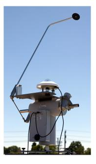
Eye has durable hardened glass window and an interface cable with connectors at both ends. Four M8 threaded holes on gearbox top for fitting available options such as the SA02/T
