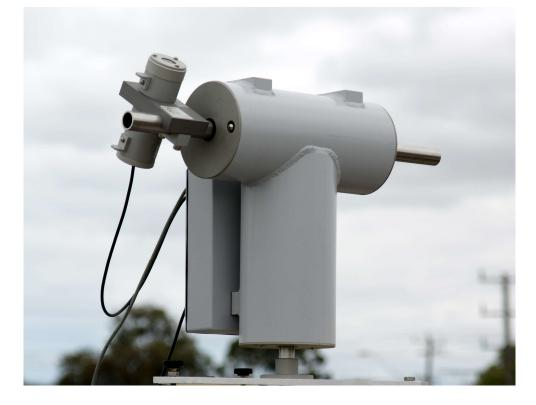
The Middleton Solar AST-02/3/3T is an active sun tracking system for solar instruments used to measure direct and diffuse irradiance. The AST-02 has a single elevation shaft. The AST-03 has two coaxial elevation shafts mechanically locked together, and the AST-03T version has two coaxial elevation shafts that are controlled separately to facilitate shade/un-shade and alignment testing.
